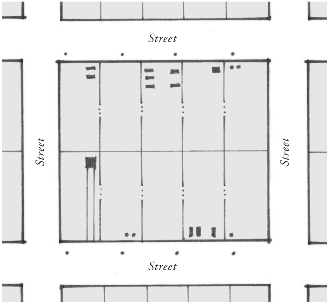
With no alleys present, many undesirable objects must occupy the front of lots.
